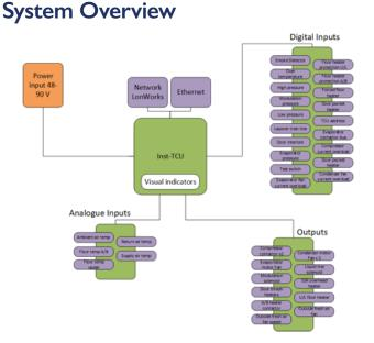
The Instrumentel TCU is a multi input / output control unit suitable for processing information from HVAC sensors and providing outputs to drive the HVAC peripherals.
