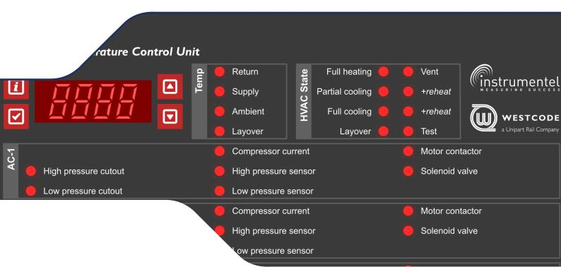
The Temperature Control Unit (TCU) system is designed to control the Heating Ventilation and Air Conditioning (HVAC) system of a rail vehicle and provide real time condition information on the current state of the HVAC operation.
